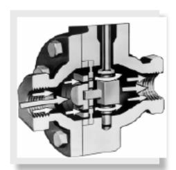
The sliding gate design provides unparalleled low flow control since the flow works with the design, not against it. In a typical globe style design the flow goes underneath the plug, working against the plug. In the sliding gate design, the flow pushes the disc against the plate, helping to hold the desired setpoint. This also enables the disc and plate to lap and clean themselves. Thus the sliding gate design, wears in instead of wearing out!
