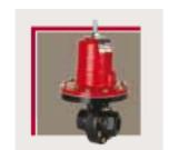
Seat Sliding gate - ANSI Class IV shutoff 1-1/2" through 2" (DN40 through DN50) Sizes Body Materials Ductile Iron, Bronze, Carbon Steel, Stainless Steel End Connections Threaded, Flanged, Socket Weld, Butt-Weld Cv (Kv) up to 70 (up to 60,2)
