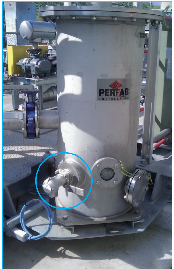
Trimod Besta level switch for low level alarm
