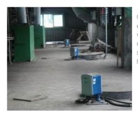
Our electromechanical system NIVOBOB NB3200 is an electromechanical system with additional advantages because of the tape version with integrated tape cleaner. Thus, the costs for maintenance is reduced. The NB3200 delivers reliable results and offers long-life and stableness also in difficult conditions. All in all, 90 units of series NB3200 have been installed in various applications.
