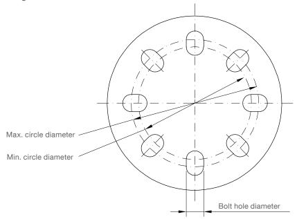
Universal flange (plane flange and Easy Aimer flange) mates with bolt hole pattern of: EN 1092-1 (PN16) ASME B16.5 (150 lb) JIS 2220 (10K)
