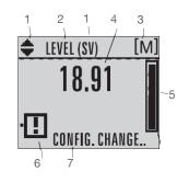
After power up the unit goes to Measurement mode.
