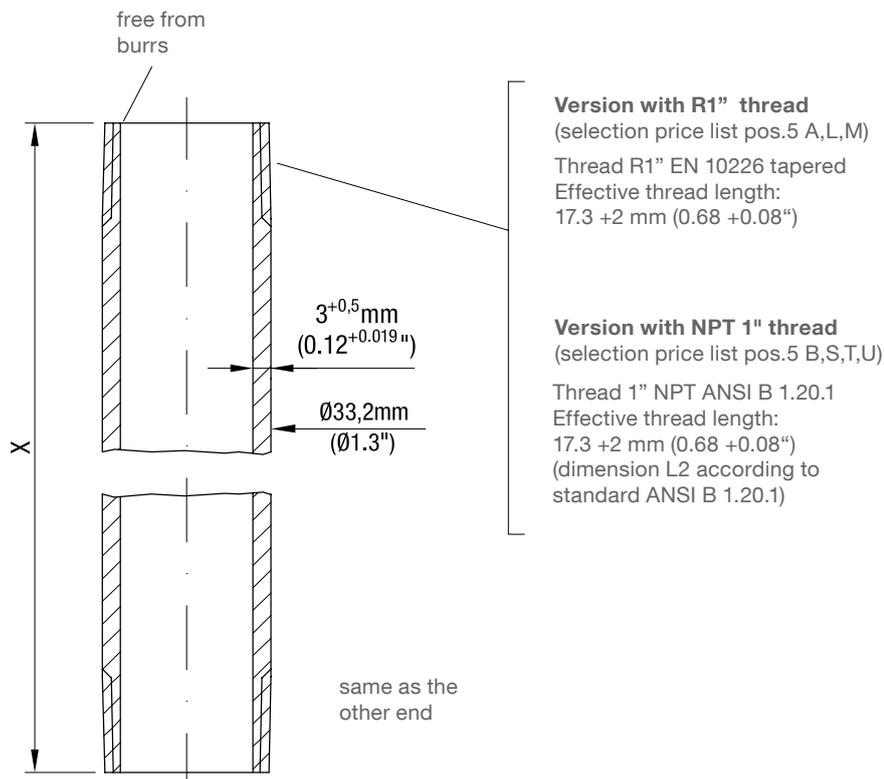
Pipe length  $X = L - 200 \text{ mm (7.9")}$
