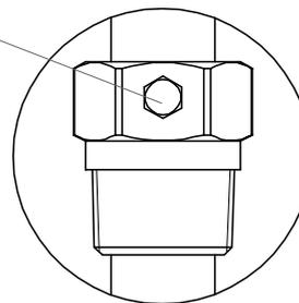
**Flange mounting** A plastic sealing must be used to tighten the flange.
