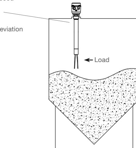
**Mounting location** Keep distance to incoming material and to the silo wall. The installation has to be done in a way, that the sensor elements cannot hit the wall of the silo. The flow of the medium and fixtures in the container must be considered. This is especially important for extension length more than 3 m (118.1“).
