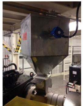
Our customer maufactures high-quality packaging solutions and therefore requires a level indicator located in a pre-bin. The indicator is responsible for a sufficient supply of the extruder with PP-regranulate. A reliable and long-lasting level indicator is therefore highly requested. The regranulate has a low DK-value of 1,7.
