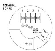
The transmitter must always be connected to earth. The transmitter must be connected with standard two-wire shielded cable. **DO NOT** run signal wiring in open trays with power wiring, or near heavy" electrical equipment (E.g. frequency controllers or heavy pumps). Shielding must always be connected at the side of the power supply.
