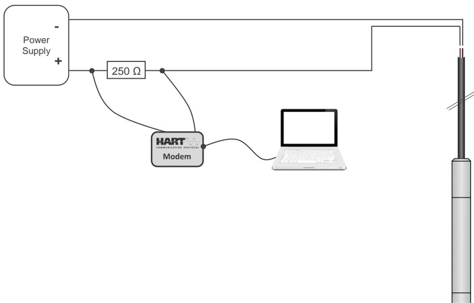
*Option 2: HART® Modem connected across the transmitter.*
