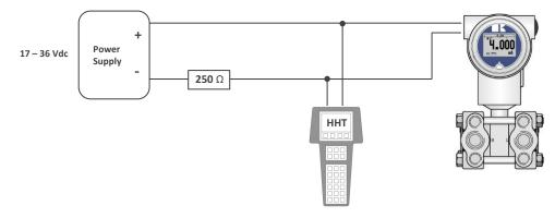
**Option 2**: HART<sup>®</sup> Handheld terminal connected across the loop resistor.
