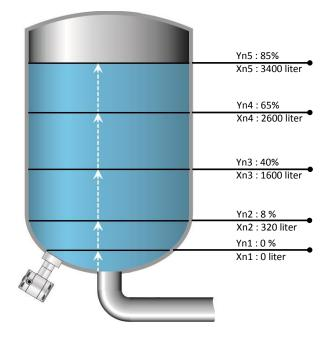
The figure above shows a tank with standard dimensions. Free linearization can applied on a wide variety of tanks with non-standard dimensions.
