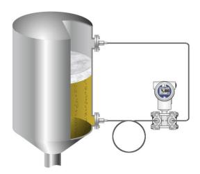
Differential pressure measurement with chemical seals.
