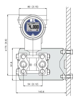
\* As standard the DP-4000 will be supplied with **two** cable entries M20 x 1,5. A cable gland can be supplied on request (extra costs).
