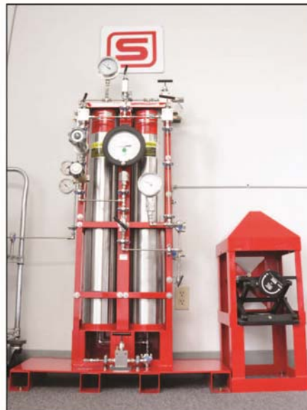
High-Pressure Accumulator Tank and Burst Test Manifold
