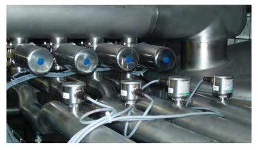
FLOW MEASUREMENT OF DEMINERALIZED WATER
