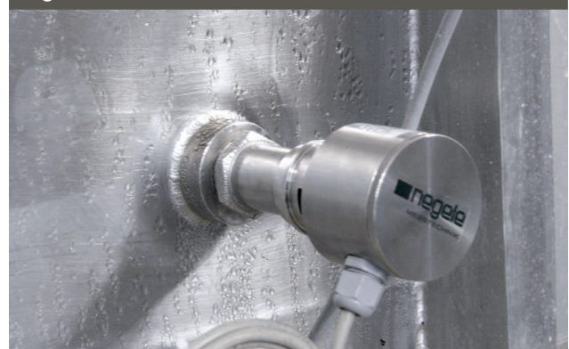
Fig. 2: Condensation on built-in level sensor
