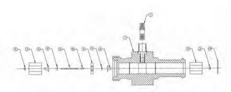
Wing Nut Meter with Tungsten Composite Sleeve Bearing (TC)
