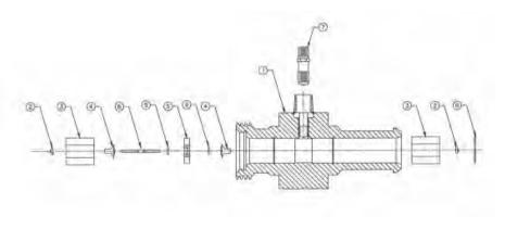
Wing Nut Meter with Ball Bearings (BB)
