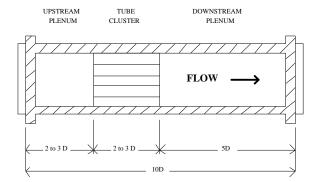
Figure 2 Typical Flow Straightener
