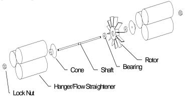
**Figure 3** Exploded View - Flowmeter Internals
