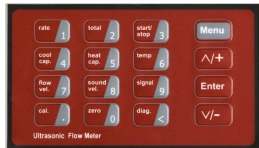
Figure 3. 16 Tactile Keys With 12 Dual-Function Keys
