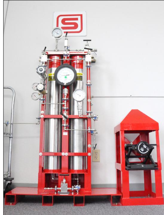
**High-Pressure Accumulator Tank and Burst Test Manifold**
