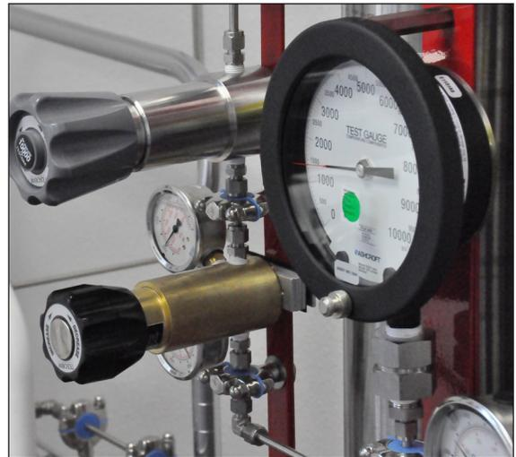
Gauge for High-Pressure Accumulator Tank Used During Calibration
