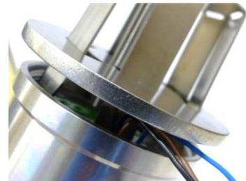
Now the puck without the display can be properly positioned and installed back in the sensor head and the wiring can be reconnected to the cable terminal. Then the large display can be mounted → see chapter 7.1 **Retrofitting the display if a display was not yet installed.**
