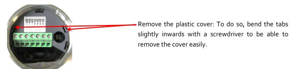
After removing the plastic cover, the large display can be inserted in the head of the sensor. The tabs (Fig. 2) must be inserted in the appropriate openings on the puck (Fig. 1). Then the display can be easily pressed onto the puck. No wiring is required.
