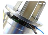
Now the puck without the display can be properly positioned and installed back in the sensor head and the wiring can be reconnected to the cable terminal. Then the large display can be mounted  $\rightarrow$  see chapter **7.1 Retrofitting the display if a display was not yet installed**.
