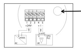
Connection plug for MPI-200-F adapter as an intermediate plug between the NSL-F electronics and the MPI-200 connection 3 (see next figure).
