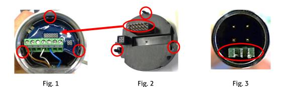
**Attention:** The connector of the programming adapter (Fig. 3) must be connected in the correct direction → the green spacer must face the cable exit (M12 connector or PG).
