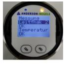
After the sensor is started, the screen saver appears in which the process values of the sensor are displayed one after the other. To reach the start page from here, press one of the two buttons briefly. Further information on operating the display can be found in the quick start manual and in the operating manual.
