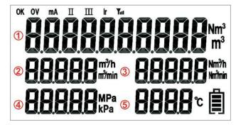
1) "OK": The running status of the flow meter. If it displays "OK", it means the flow meter is working well. if it display"ERR", please check the self check menu for more information.
