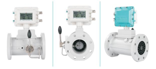
Gas turbine flow meter take into account the compressibility of gases, and the correlation between volume, temperature and pressure of the medium. To convert Process Work Condition medium to Standard Condition, temperature and pressure sensors are added to track temperature and pressure changes of the measuring medium.
