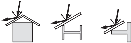
Fig. 15: Cover flat, large-area profiles with deflectors
