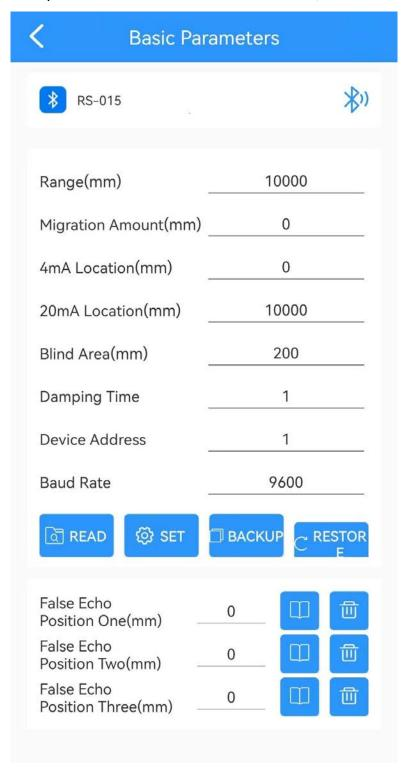
Set the "Range" according to the working conditions and directly click the number input box behind to modify it.
