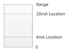
As shown in the figure, when the liquid level is lower than 4mA Location, the main interface displays the liquids level as 0; when the liquid level is higher than the 20mA location, the main interface displays the liquid level value as the value of 20mA location.
