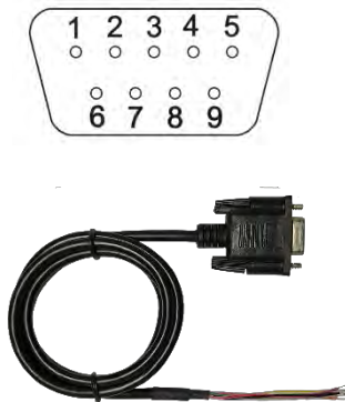
Figure 3.3: MF5100 socket and cable
